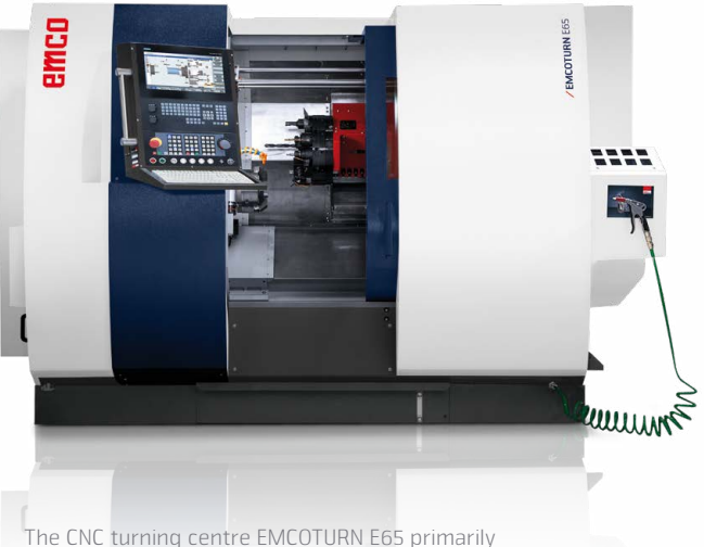
The CNC turning centre EMCOTURN E65 primarily produces screw cores for GF Casting Solutions. This makes it possible to produce spare parts at a high level and at high speed.
