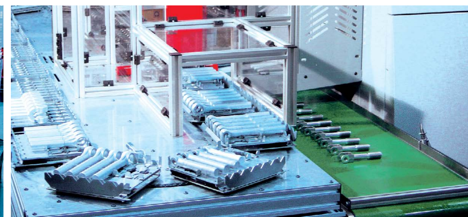
20-station pallet magazine with customer-specific pallets
