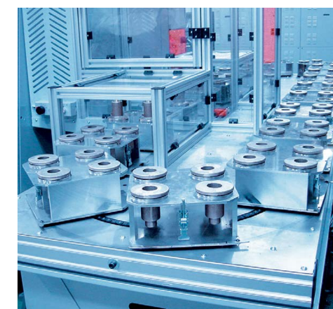
4-station pallet attachment for valve caps
